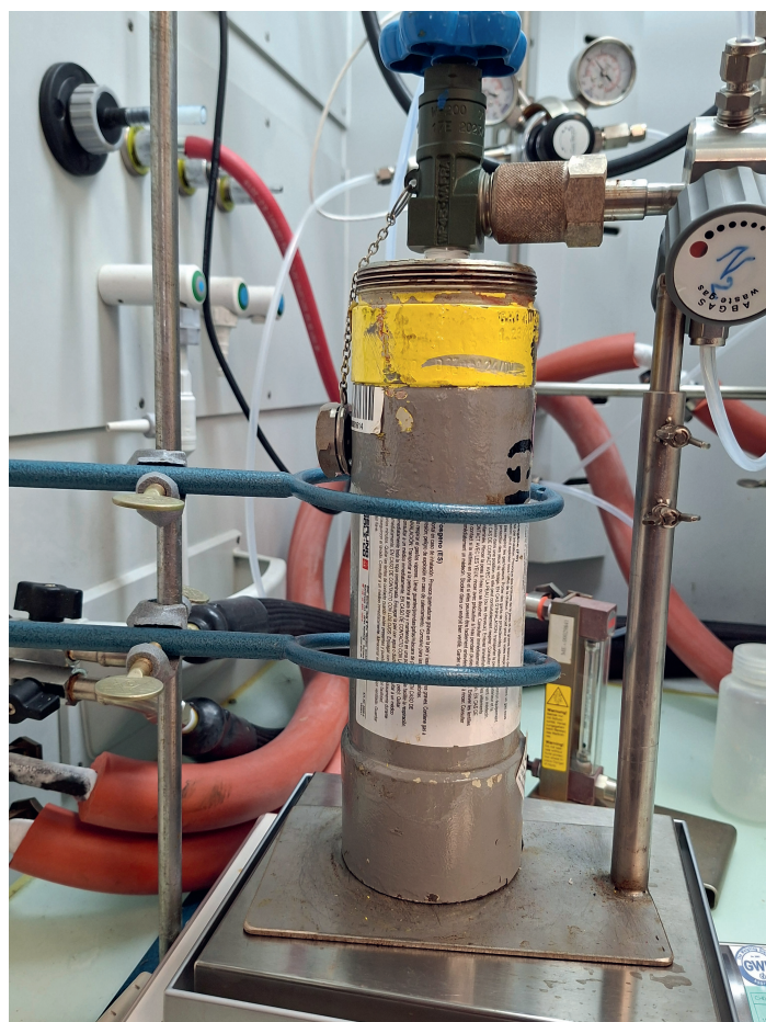
Fig. 5. 1.2 kg Phosgene bottle. The consumption over the dosing time can be monitored using the scale below.
